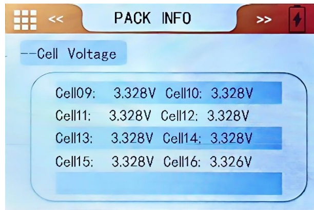
Figure 6-4-4 Cell Voltage Information Interface 2
